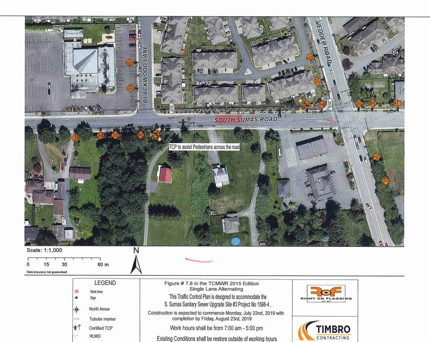
This traffic plan is based on a maximum 50 Km speed zone
